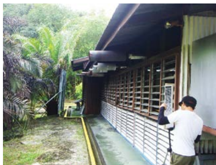
Dark smoke observation using the Ringelmann Chart at Belaga
