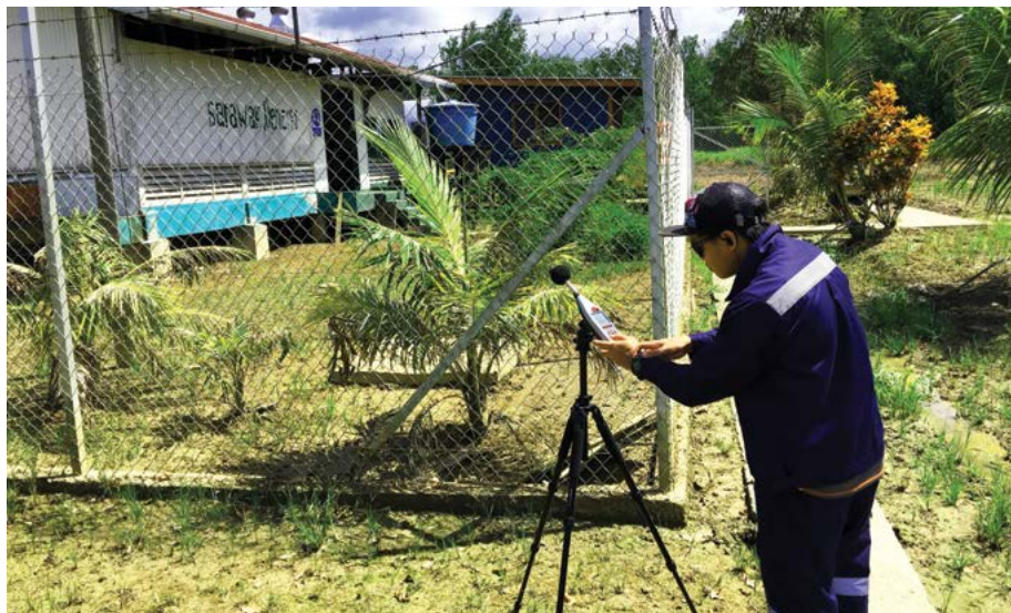
Boundary noise monitoring at the perimeter fencing at Banting, Sri Aman. The allowable noise level for most power stations is 65 dBA at all times
