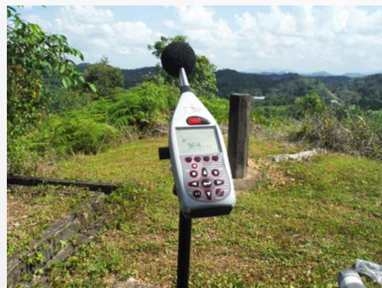
Boundary noise monitoring at the perimeter fencing. The allowable noise level for most power station is 65 dBA at all times
