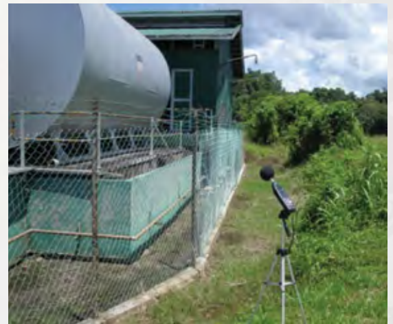
Boundary noise monitoring at the perimeter fencing. The allowable noise level for most power station is 65 dBA at all times
