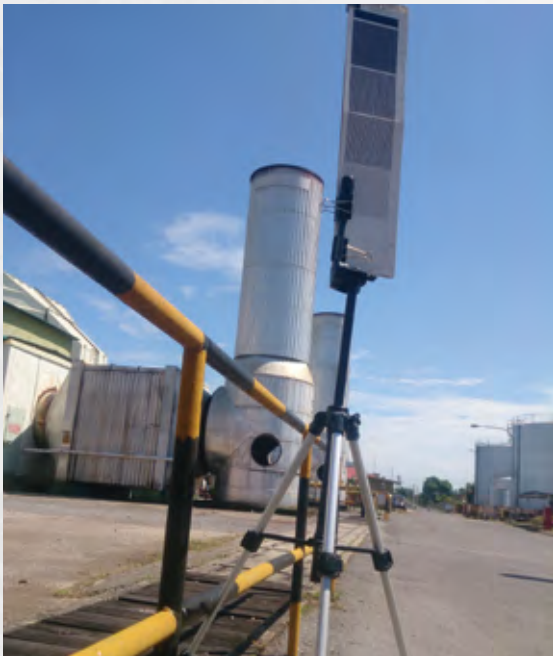
Dark smoke observation using the Ringelmann Chart. Smoke must not be darker than No. 120
