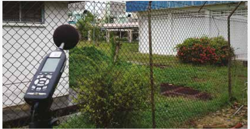
Boundary noise monitoring at the perimeter fencing. The allowable noise level for most power stations is 65 dBA at all times
