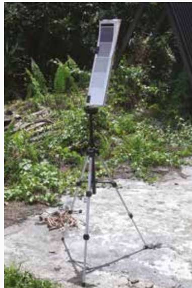
Dark smoke observation using the Ringelmann Chart. Smoke must not be darker than shade No. 120
