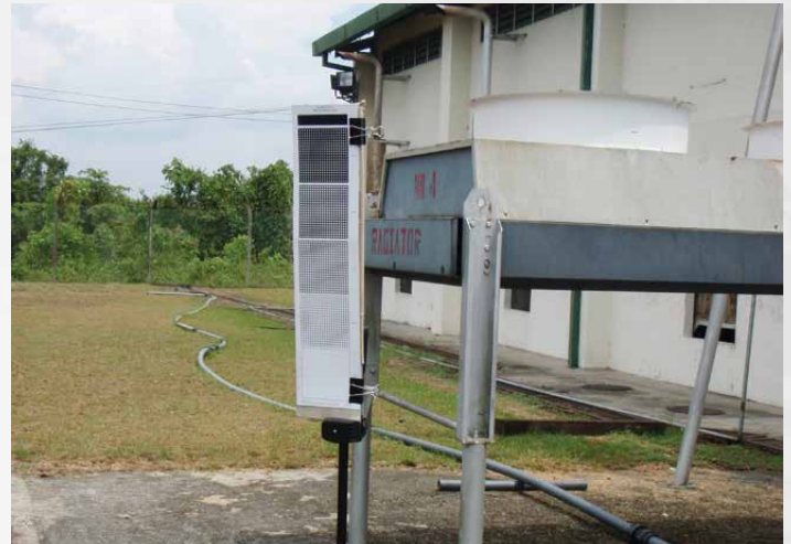
Dark smoke observation using the Ringelmann Chart. Smoke must not be darker than shade No. 120
