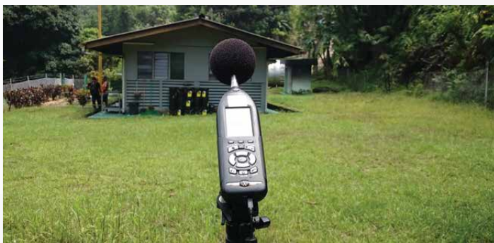
Boundary noise monitoring at the perimeter fencing. The allowable noise level for most power stations is 65 dBA at all times
