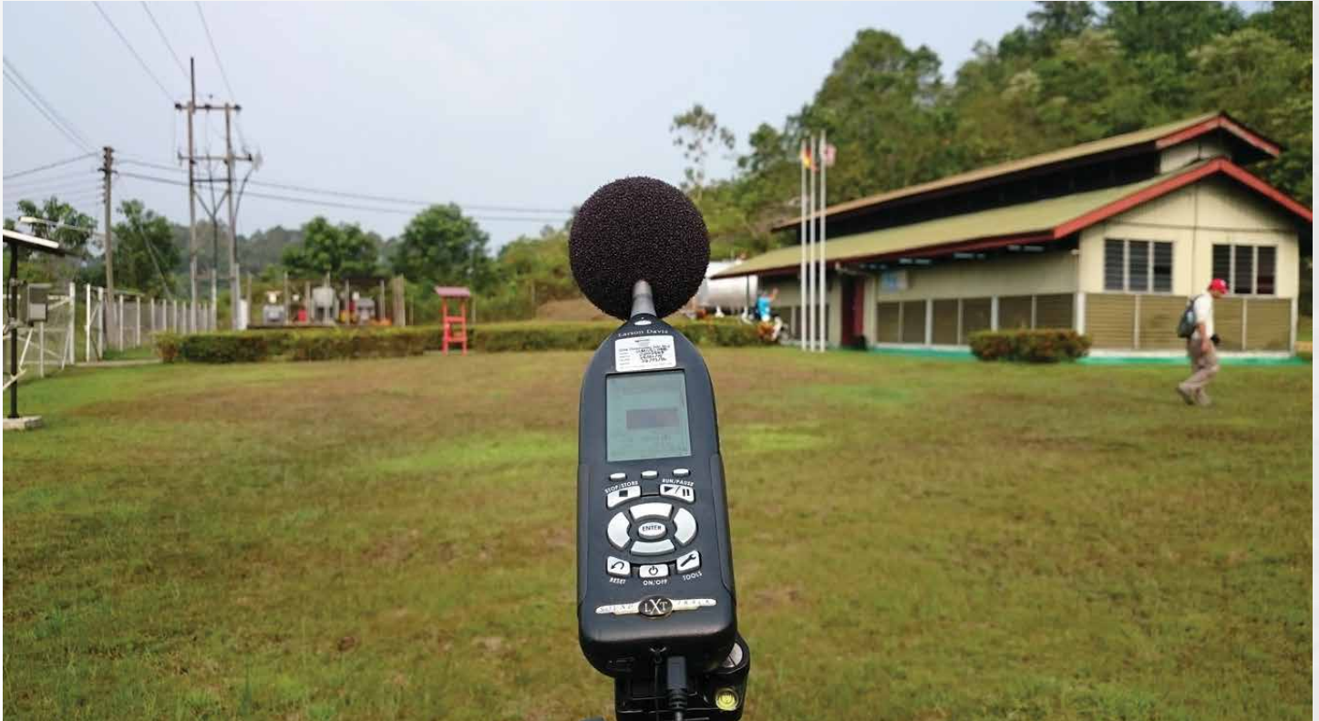
Boundary noise monitoring at the perimeter fencing. The allowable noise level for most power stations is 65 dBA at all times
