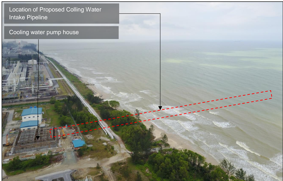
Figure 4: Ariel photograph of cooling water pump house and proposed cooling water intake pipeline (source: Sinohydro)
