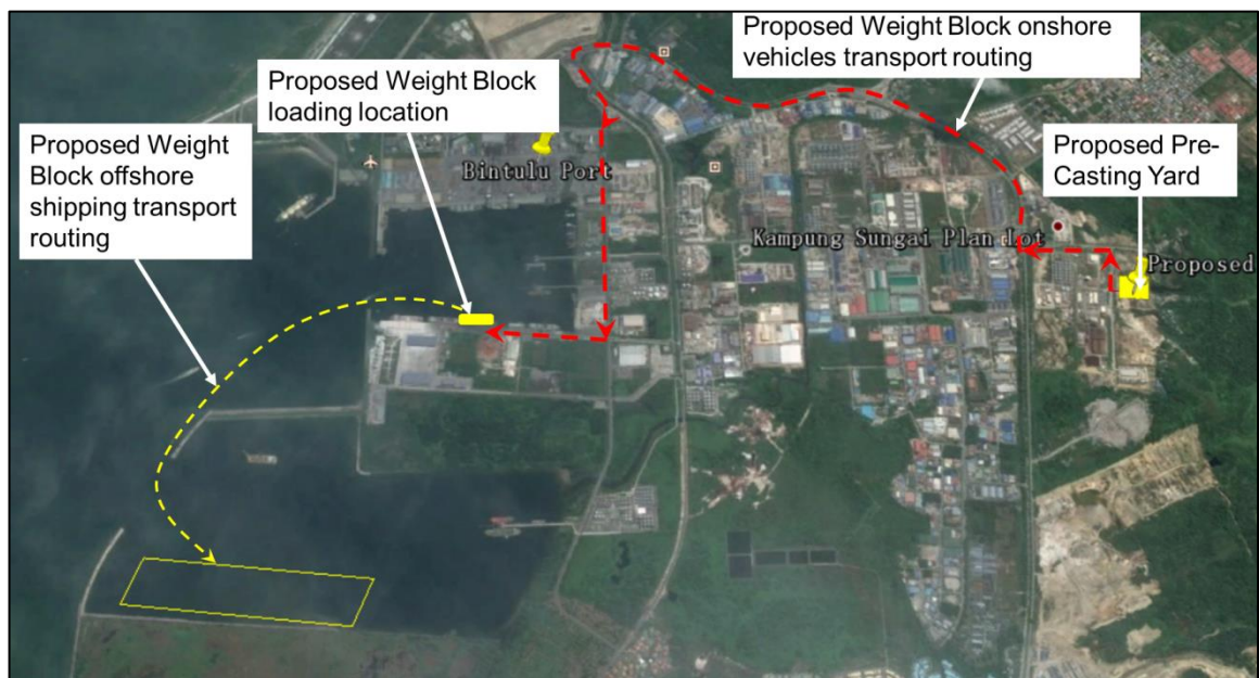
Figure 13: Proposed barge route for transportation of weight balancing blocks (source: PowerPoint for HDPE Pipeline Transportation, Storage and Assembly received on 12 th February 2018 from Sinohydro)
